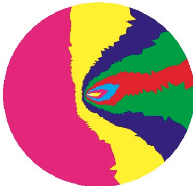
Figure 3.3. 8-way partitioning of the RAE2822 grid (figure 3.1) from the Gibbs-Poole-Stockmeyer reordering (Courtesy Bruner, C.W.S. [29])
