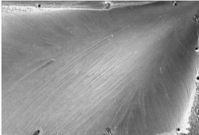
Figure 6.3. Oil flow pattern on front part of bridge deck of GSS for 30° yaw case
