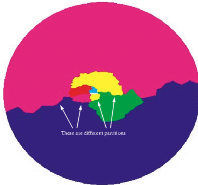
Figure 3.2. Typical 8-way partitioning of the RAE2822 grid (figure 3.1) using a graph partitioning algorithm. The colors correspond to different computational domains (or partitions). (Courtesy Bruner, C.W.S. [29])
