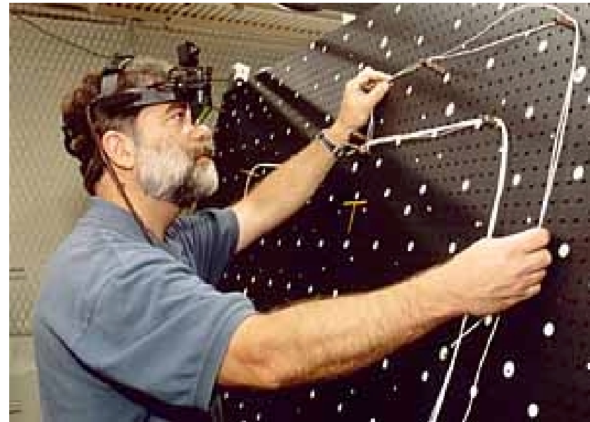
VR HUDset used in the wire shop to connect the wires by showing an image of the circuit and information about type of wire to be used (Boeing, US)
