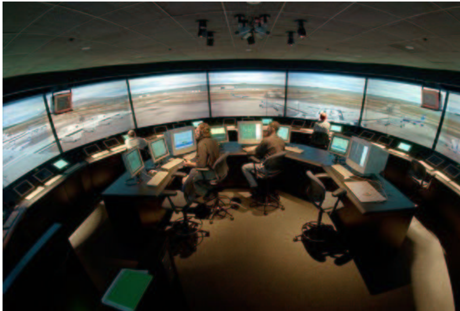
Figure 2.6. An IVE system for ATC: NASA FutureFlight Central's tower [64]
