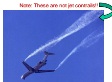
Wake-vortex generated by a Boeing 727 (Courtesy NASA)
