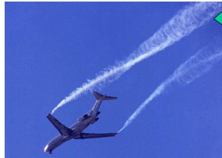
Wake-vortex generated by a Boeing 727 (Courtesy NASA)
